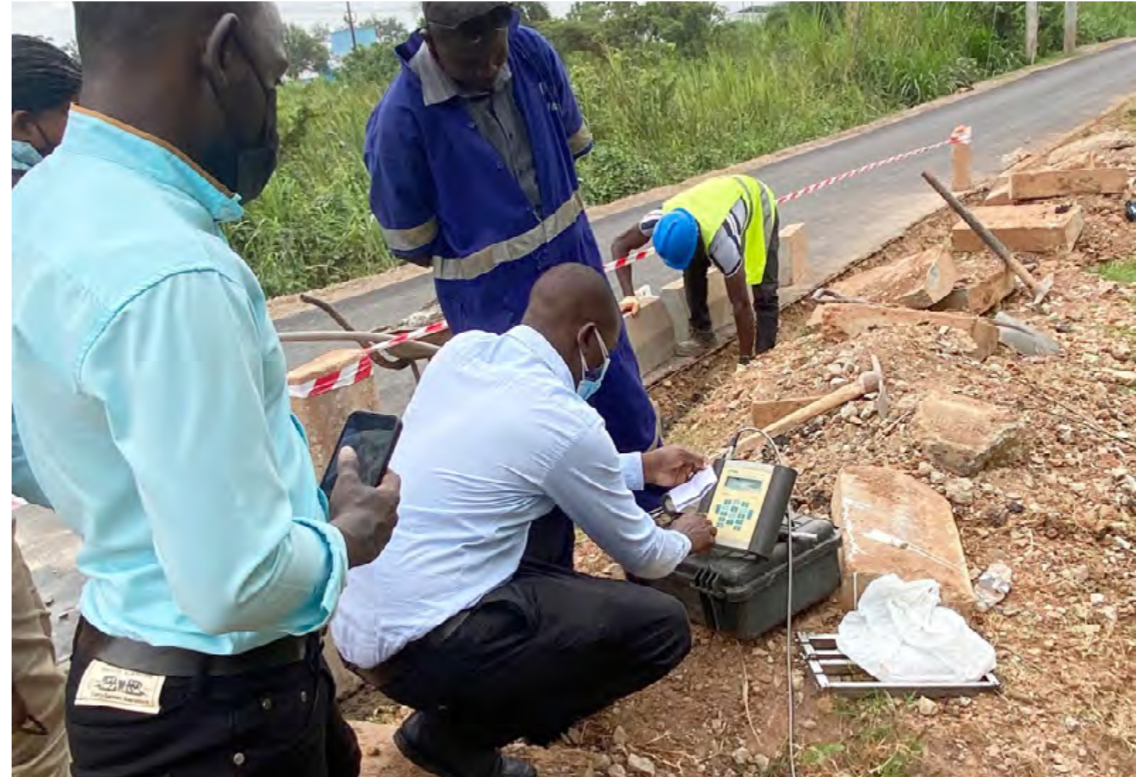
Uganda – An online measurement is being carried out in Kampala with the support of Short Term Expert Roy van der Knaap from Evides Waterbedrijf. With a clamp-on water meter, the flow rate of a transport pipeline is measured to validate the accuracy of the existing service meter.
